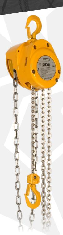
With a weight of just up to 28 kg KITO's CF model is ideal for its ease of handling and portability. The KITO CF is unique with its single reduction gearing that results in lifting speeds up to 28% faster than typical manual chain hoists. Moreover it is built with double pawl springs, and heavy duty heat-treated pinion and gears. The gear shafts with ball bearings minimize friction to guarantee ease of operation.
