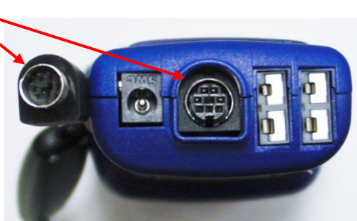
“D” Shaped mini-DIN connector
